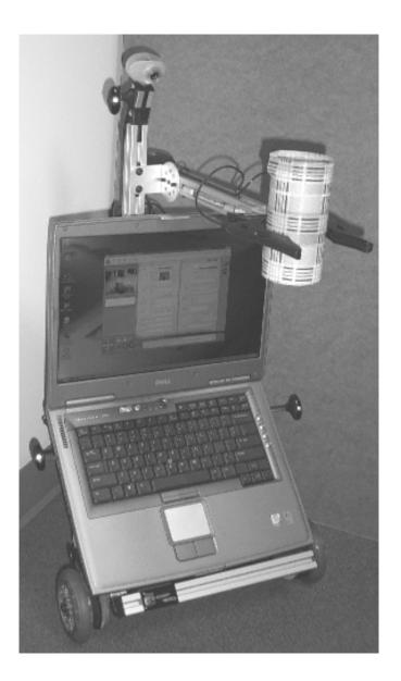
Figure 2. An ER1 robot, configured its gripper in a high location (holding a cup), its camera (on the top of the stalk), and the interface that is mirrored on another computer (shown in Figure 3) that controls the robot remotely.
