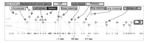
Figure 5: Example of lane change on a motorway (screenshot with text labels added at the top).
