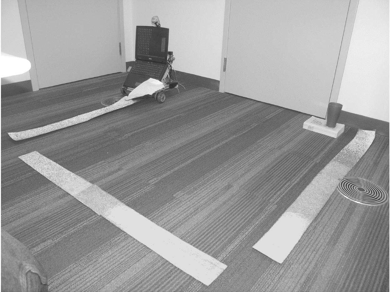
Figure 4. The physical task environment for the human users. The robot's path for human subjects was red on a blue-gray striped floor; the model drove on a table that provided greater image contrast using a black path on a white tabletop.
