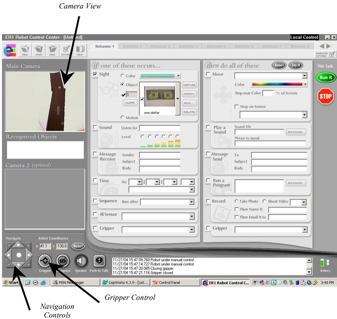
Figure 3. The HRI interface that users saw when driving the ER-1 robot remotely.
