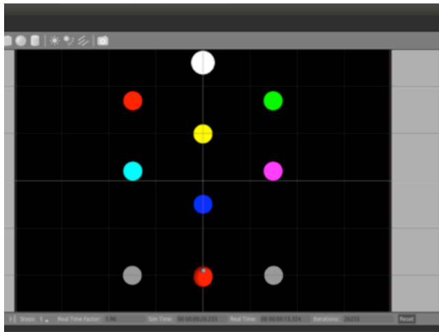
Figure 1: Gazebo robot simulator. Screenshot of Gazebo simulator showing the prototypical top view of a foraging task used to benchmark DAC with colored patches on the floor and a source of light represented by a bigger white patch on top of the screen.
